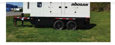
Doosan Portable Power's G325 is the first in a series of new models that meet Tier 4i emissions standards. Photo courtesy Dooson Portable Power.
