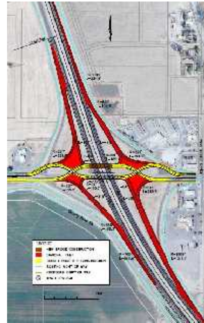
Concept 3: Diverging Diamond Interchange
