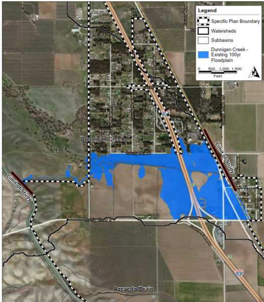
Exhibit 5.10 Dunnigan Creek Existing Floodplain
