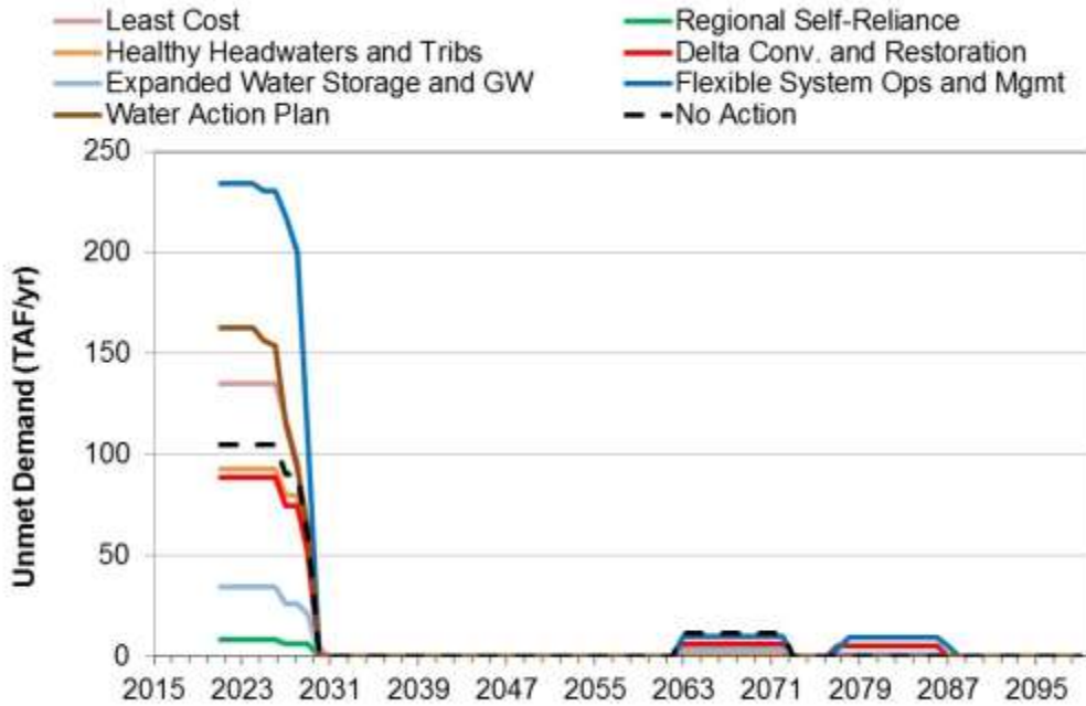
Figure 7-3b. 10-year running average of unmet demand in the Sacramento River System in each adaptation portfolio in the Central Tendency climate/Current Trends socioeconomic scenarios.
