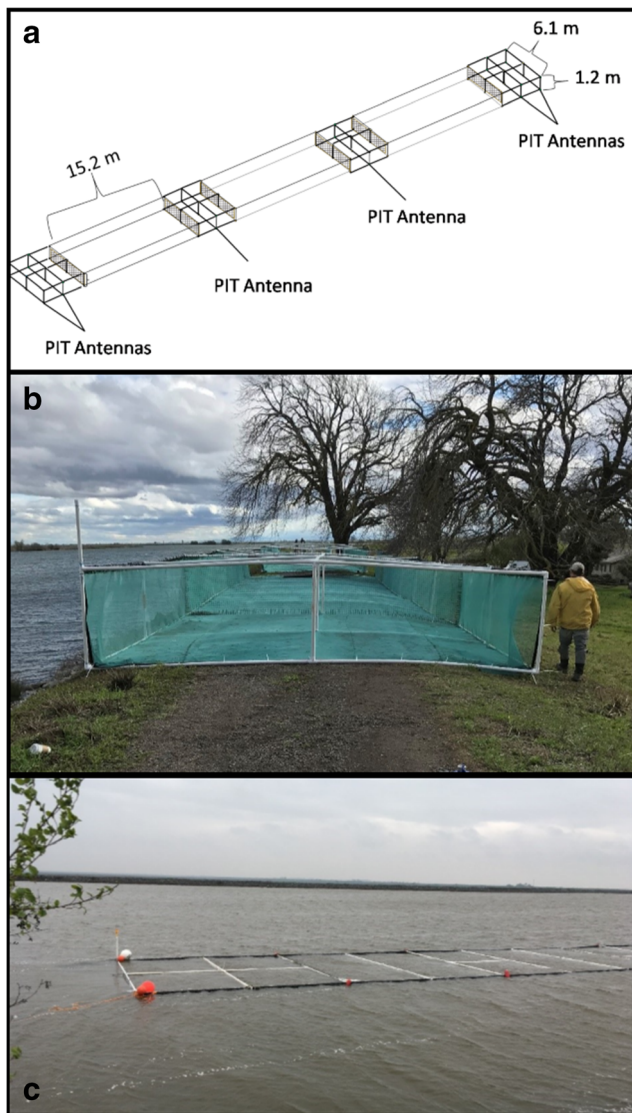
Fig. 2 Diagram of the experimental enclosure with size measurements (top panel), and pictures of the enclosure under construction (middle panel) and deployed during the experiment (bottom panel)
