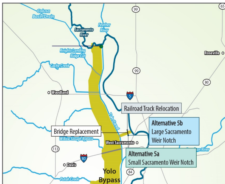
Figure 3-7. Initial Alternative 5: Sacramento Weir Notch
