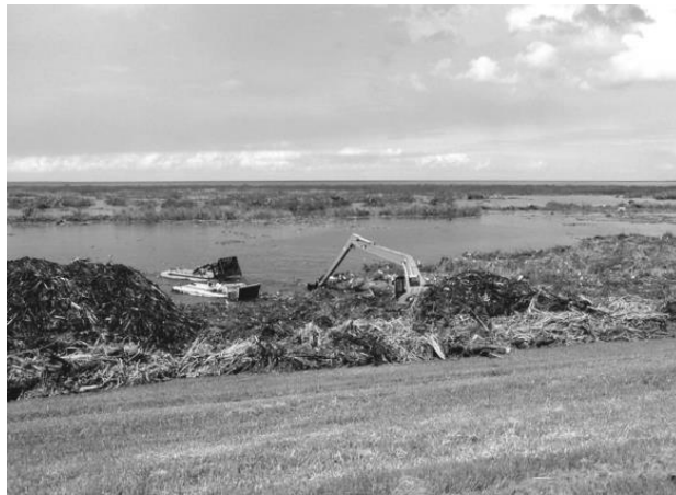
Figure 11.8. Pushing aquatic plants to shore for harvesting by track hoe. Photo credit: Center for Aquatic and Invasive Plants, University of Florida, Gainesville.
