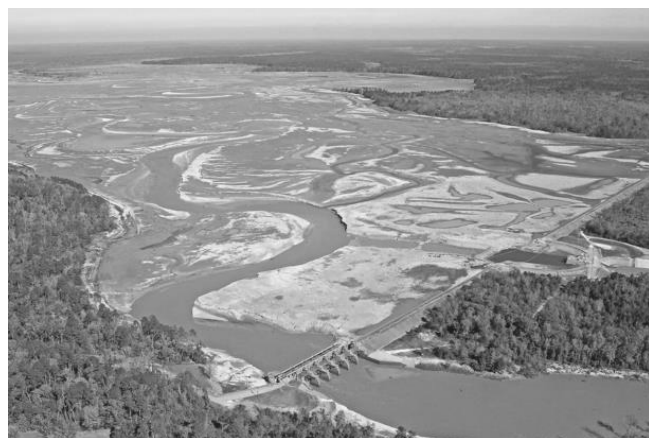
Figure 11.9. Drawdowns to control nuisance aquatic vegetation on B. A. Steinhagen Lake reservoir, Texas, were successful only when coordinated with prognostic of bitterly cold temperatures. Photo credit: U.S. Army Corps of Engineers, Town Bluff Project.
