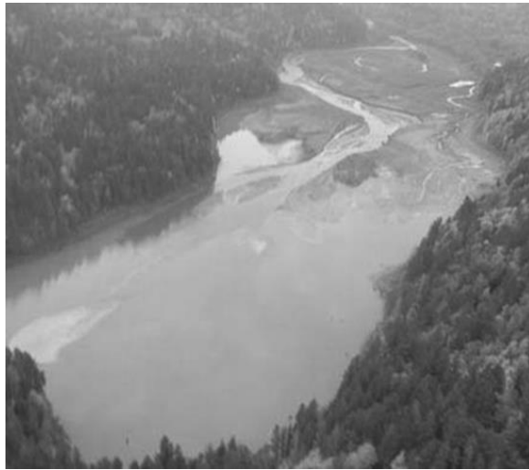
Figure 3.16. The sediment built up in the upper end of Lake Aldwell, impounded by the Elwha Dam, Washington, was exposed by a drawdown, eroded by the river, and flushed downstream. The dam was eventually removed, and the Elwha River flowed freely through the site by March 2012. Photo credit: B. Cluer.
