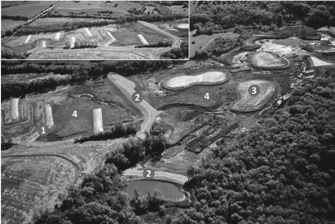
Figure 4.3. Constructed retention cells and wetland complexes in the 4,700-ac watershed of Iron Horse Trail Lake reservoir, Nebraska. The inset in the top left shows Lores Branch approaching the complex. The complex slows down flows and allows expansion into wetlands to remove sediment and nutrients approaching the reservoir. 1 = channel training and maintenance access berms; 2 = sediment retention dikes; 3 = islands created from in-lake sediment spoils; 4 = wetlands. The top of the berms are lower than the top of the sediment retention dikes, and are designed to train the normal stream inflows to meander during normal flows and small rain events, but will be overtopped at high flows. Wetland vegetation will grow around the berms. During drawdowns the berms provide access for heavy equipment to remove deposited sediment. Photo credit: M. Porath, Nebraska Game and Parks Commission, Lincoln.
