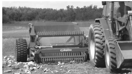
Figure 5.17. Rock often found scattered along the regulated zone can be collected with a rock picker and piled to construct stone reefs and/or shore reinforcements. Photo credit: Highline Manufacturing Ltd., Vonda, Saskatchewan.
