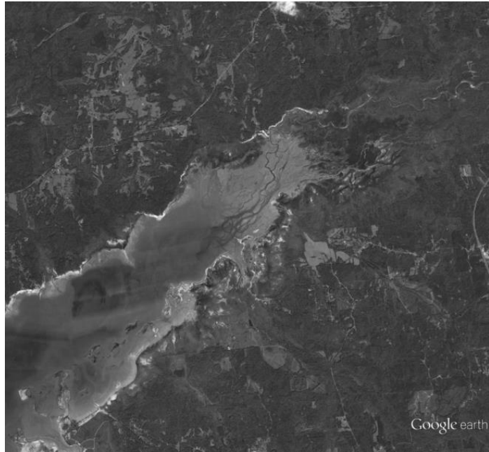
Figure 3.2. Sedimentation delta formed in the upper end of Sardis Lake reservoir, Mississippi. This reservoir impounds 32,500 ac at normal pool and is over 75 years old. Photo credit: Google Earth.
