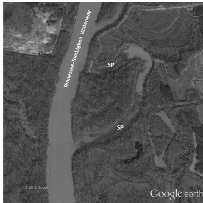
Figure 9.2. Bendway (channel of the original river) isolated from the uplake section of Columbus Lake reservoir, Mississippi. The river was channelized to facilitate navigation, and bendways were cut off on both sides of the new navigation channel. Cutoff bendways trap sediment that creates sediment plugs (SP) near their entrance and eventually become seasonally or permanently isolated from the reservoir unless weirs are installed to increase flow through the bendway or closing structures prevent flow into the bendway. Photo credit: Google Earth.
