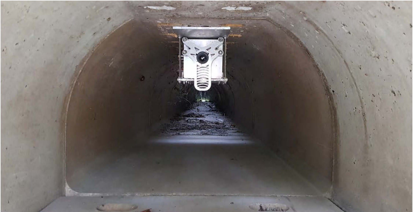
Figure 66: Cameras have become an integral part of small wildlife passage studies. In this passage, a short-focusing camera with night vision has a wide-angle infrared time-lapse. It takes four pictures per minute as a sampling technique that misses few amphibians. Image: HCI Ltd.
