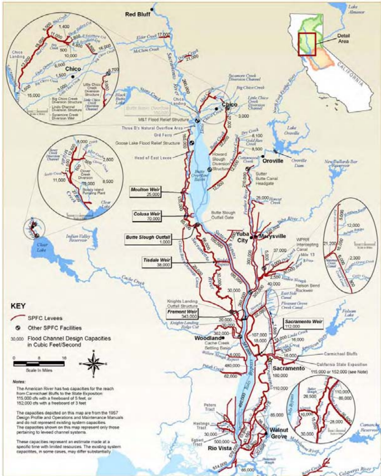
Figure 3-2. Design Flood Flow Capacities Within the Sacramento River, Bypasses, and Major Tributaries and Distributaries in the Sacramento River Basin
