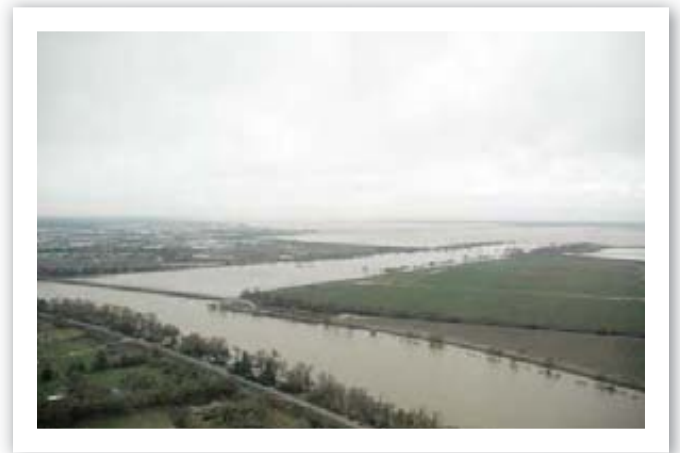
The design flood flow capacity of the Sacramento River upstream from Sacramento Weir is 107,000 cfs
