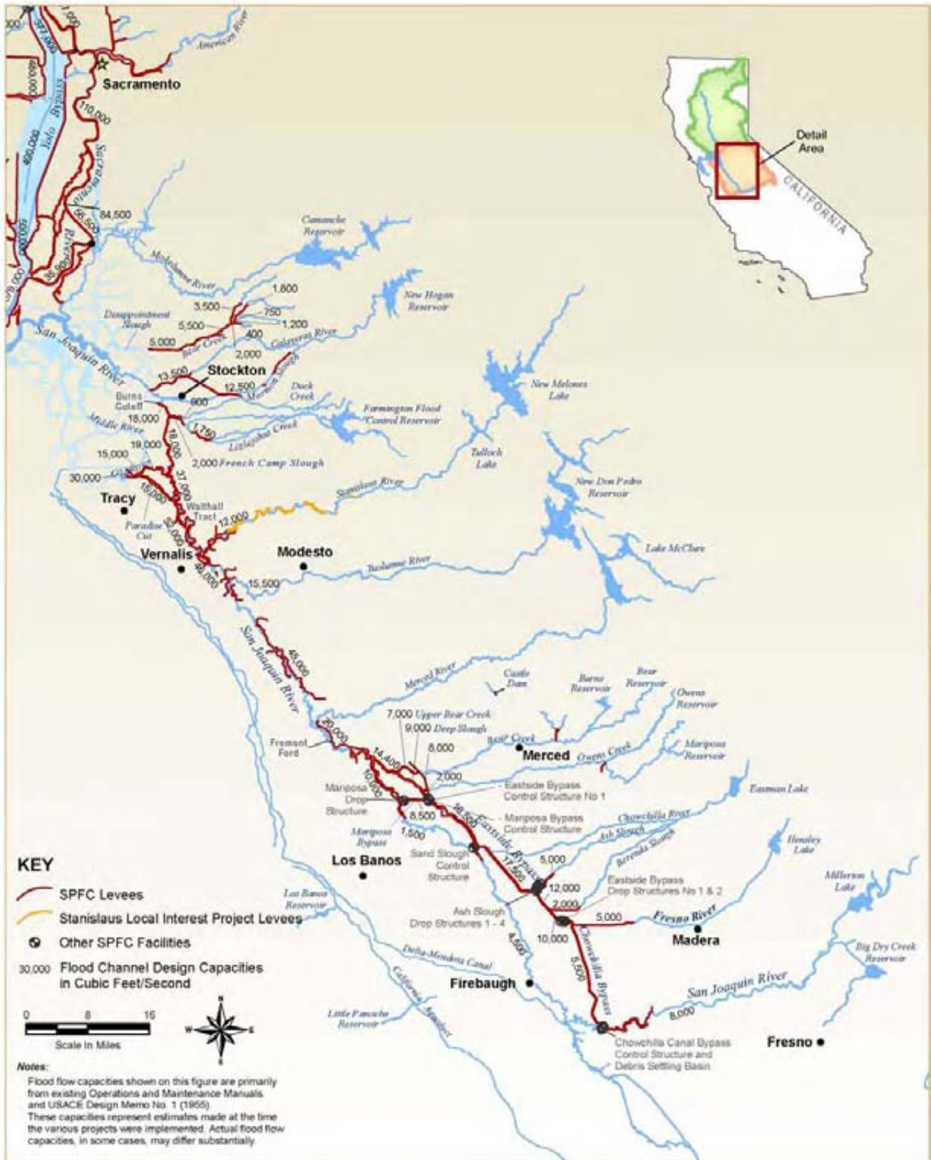
Figure 3-3. Design Flood Flow Capacities Within the San Joaquin River, Bypasses, and Major Tributaries and Distributaries in the San Joaquin River Basin
