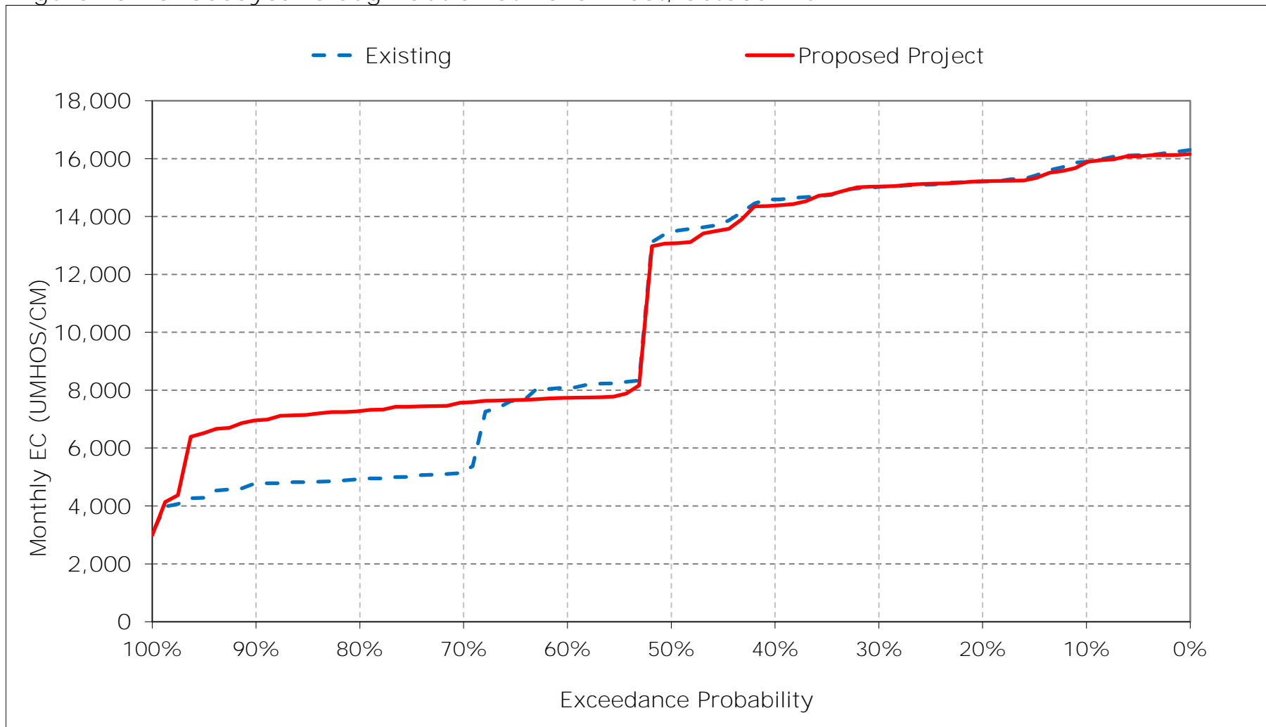
Figure 25-16. Goodyear Slough Outfall at Naval Fleet, October EC
