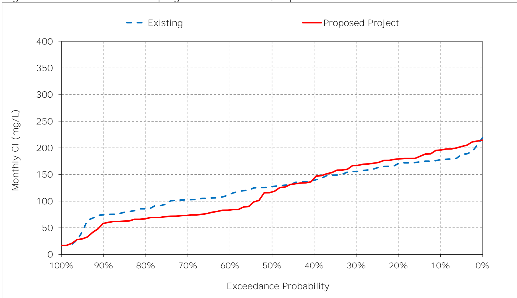
Figure 9-15. Contra Costa Pumping Plant #1 Chloride, September CI
