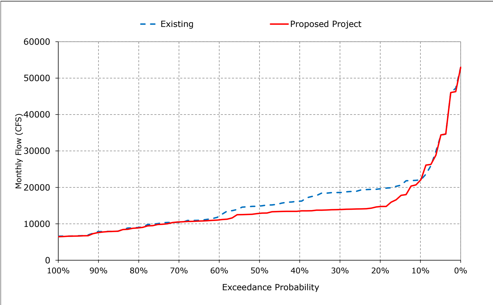
Figure 1-8. Sacramento River Flow at Freeport, November
