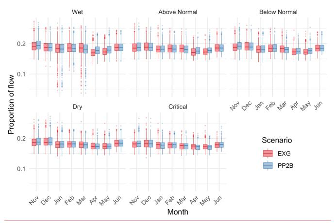
Figure 5.3-64. Box and Whisker Plots of the Proportion of Flow Entering the Middle River Junction with the San Joaquin River. Proportions were summarized for Refined Alternative 2b (PP2B) and Existing Conditions (EXG) scenarios between November and June for each water year-type
