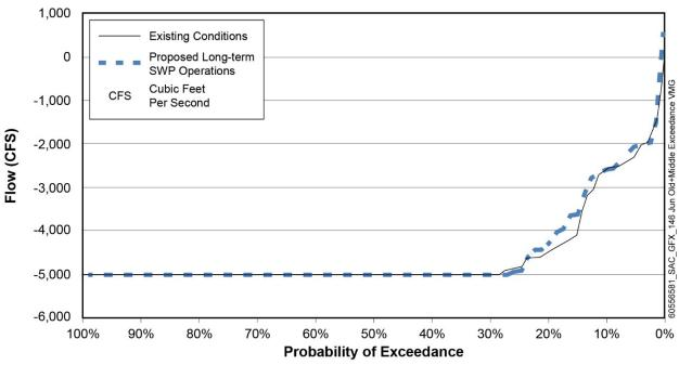
Source: <DWR\_ITP\_Trend\_Reporting\_rev18cy\_DV4\_CALSIM\_20190821\_\_Existing\_PP.xlsm> Figure 4.4-53. Mean Modeled Old and Middle River Flow, June
