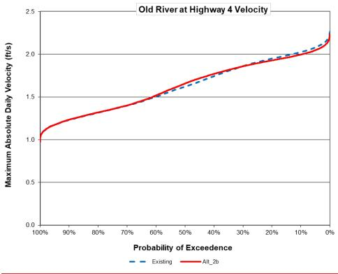
Source: <marin\_absDmax.dss, marin\_absDmax20200107.dss> Figure 5.3-35. Modeled Maximum Absolute Daily Velocity in Old River at Highway 4, June–November
