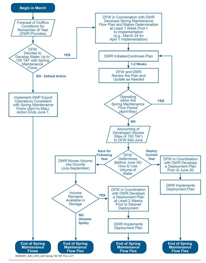
Figure 5.3-1 - Decision Points for Spring Maintenance Flow and Potential Use for Development up to 150 TAF for Deferred Flow Actions
