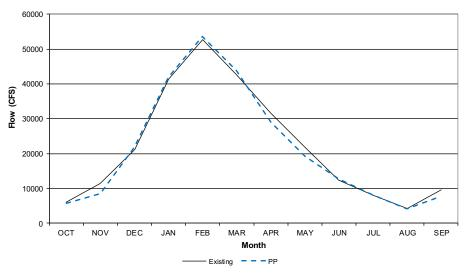
Figure 4.4-8687. Monthly Average Simulated Total Delta Outflow under the Proposed Project and Existing Conditions CalSim II Modeling Scenarios
