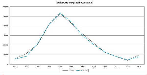
Figure 5.3-73. Monthly Average Simulated Total Delta Outflow under Refined Alternative 2b and Existing Conditions CalSim II Modeling Scenarios
