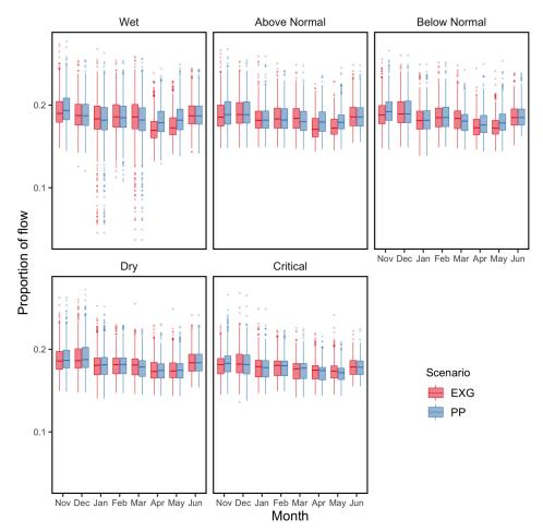
Figure 4.4-7778. Box and Whisker Plots of the Proportion of Flow Entering the Middle River Junction with the San Joaquin River. Proportions were summarized for the Proposed Project and Existing Conditions scenarios between November and June for each water year-type
