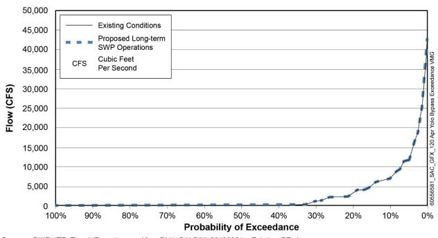
Source: <DWR\_ITP\_Trend\_Reporting\_rev18cy\_DV4\_CALSIM\_20190821\_\_Existing\_PP.xlsm> Figure 4.4-20. Mean Modeled Flow Through Yolo Bypass, April
