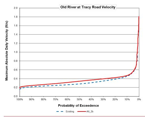
Source: <marin\_absDmax.dss, marin\_absDmax20200107.dss> Figure 5.3-31. Modeled Maximum Absolute Daily Velocity in Old River at Tracy Road, June–November
