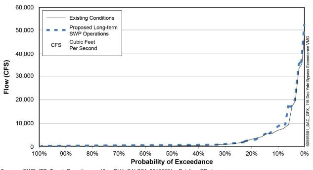
Source: <DWR\_ITP\_Trend\_Reporting\_rev18cy\_DV4\_CALSIM\_20190821\_\_Existing\_PP.xlsm> Figure 4.4-16. Mean Modeled Flow Through Yolo Bypass, December
