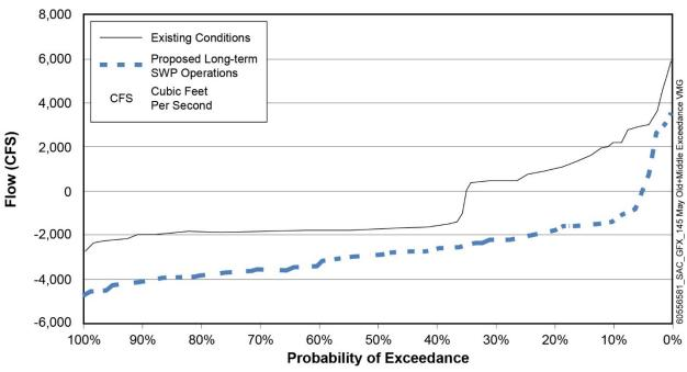
Source: <DWR\_ITP\_Trend\_Reporting\_rev18cy\_DV4\_CALSIM\_20190821\_\_Existing\_PP.xlsm> Figure 4.4-52. Mean Modeled Old and Middle River Flow, May
