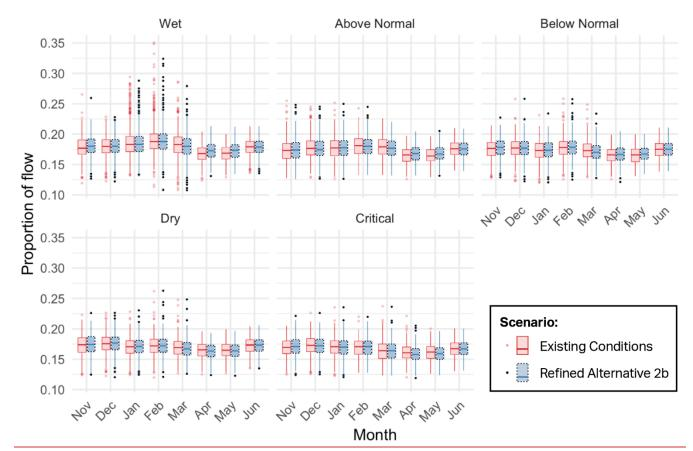
Figure 5.3-65. Box and Whisker Plots of the Proportion of Flow Entering the Old River Junction with the San Joaquin River. Proportions were summarized for Refined Alternative 2b and Existing Conditions scenarios between November and June for each water year-type
