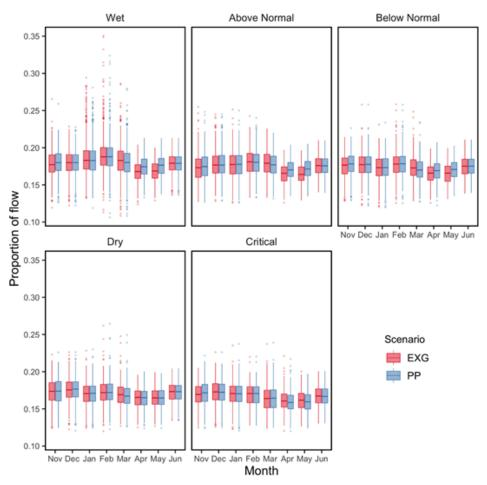
Figure 4.4-7879. Box and Whisker Plots of the Proportion of Flow Entering the Old River Junction with the San Joaquin River. Proportions were summarized for the Proposed Project and Existing Conditions scenarios between November and June for each water year-type
