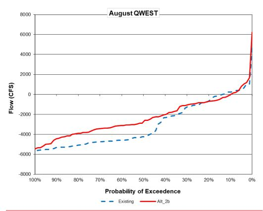
Source: <ITP\_Proposed Project\_0819.dss> and <ITP\_Alt2B\_0102\_lastCycle.dss> Figure 5.3-286. Mean Modeled QWEST Flow, August
