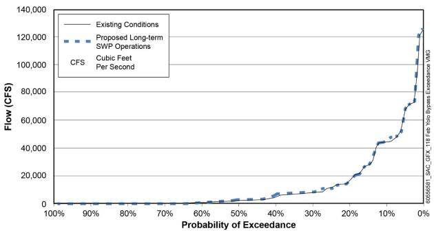
Source: <DWR\_ITP\_Trend\_Reporting\_rev18cy\_DV4\_CALSIM\_20190821\_\_Existing\_PP.xlsm> Figure 4.4-18. Mean Modeled Flow Through Yolo Bypass, February
