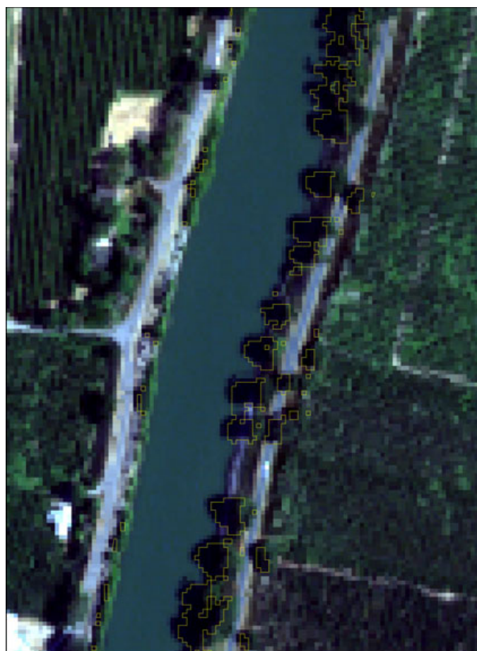
FIGURE 3. True-Color Subset of a Validation Aerial Image (HyMap) with the Boundaries of r.sun Modeled Shadows for the Same Date and Time as the Aerial Overflight Outlined in Yellow. The actual shadows can be seen projecting roughly west from the shoreline. Pixel sizes are 3 m.
