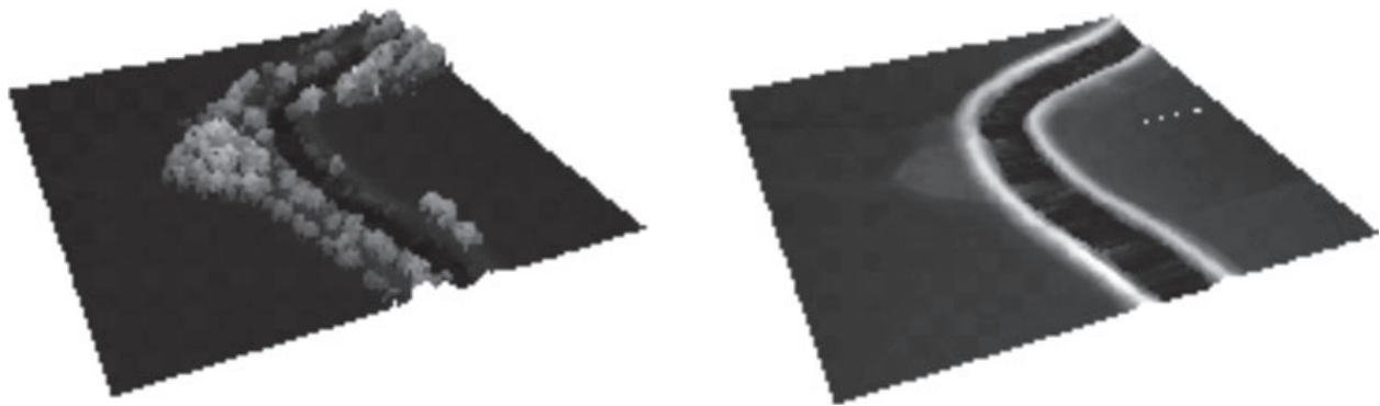
FIGURE 1. Left: LiDAR First Return Raster of a Wooded River Bend with Trees (current conditions); Right: Bare Earth Raster of the Same River Bend (treeless Delta). The images are 500 m \times 500 m. Brighter values indicate higher elevation.
