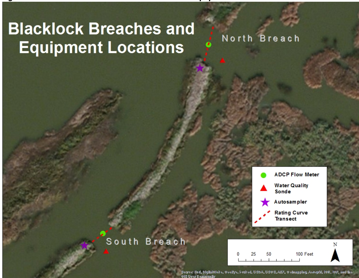
Figure 15 – Blacklock Tidal Wetland Breaches and Equipment Locations
