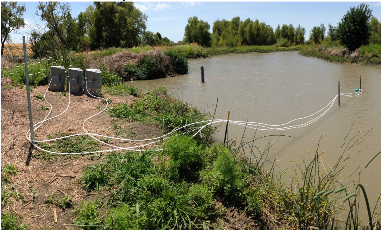
Figure 4 – Autosamplers deployed at the Yolo Wildlife Area Tidal Wetland with PTFE suction lines attached to stakes and a float in the water
