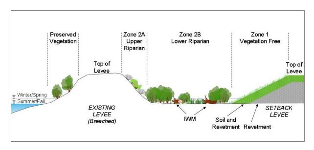
Figure 8. Conceptual design of a setback levee with revegetation and in-stream woody material enhancements.
