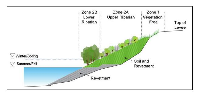
Figure 4. Design 1 – Bank fill rock slope with revegetation.
