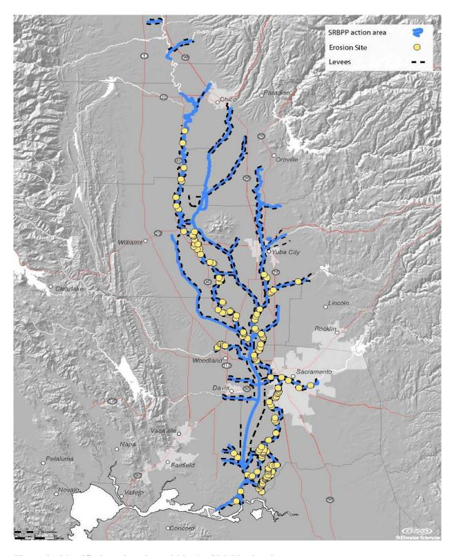
Figure 2. Identified erosion sites within the SRBPP planning area.
