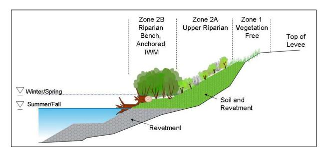
Figure 6. Design 3 – Low riparian bench with revegetation and anchored in-stream woody material enhancements *above and below* the summer/fall waterline upstream of RM 30.
