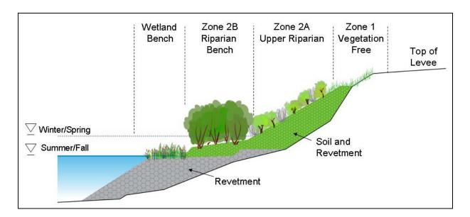
Figure 7. Design 4: Delta smelt design – Low riparian and wetland benches with revegetation downstream of RM 30.
