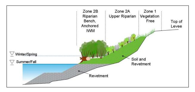
Figure 5. Design 2 – Low riparian bench with revegetation and anchored in-stream woody material enhancements *above* the summer/fall waterline upstream of RM 30.
