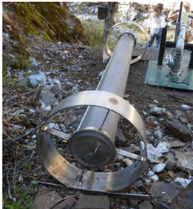
4890 4891 Figure 10-10. Typical end-of-pipe screen equipped with “wagon wheels” to elevate the screen 4892 off the stream bottom
