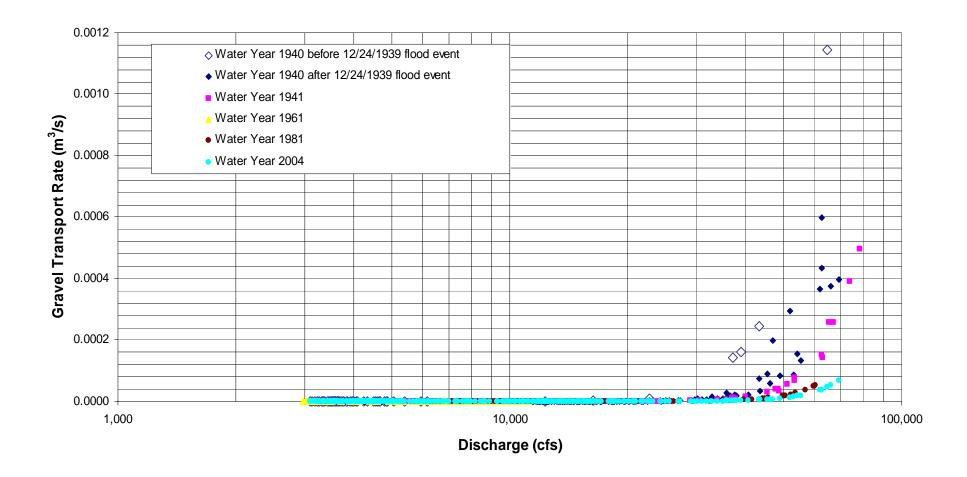
Figure 4.2-18. Modeled relationship between flow and sediment transport for RM 294 at selected times after Shasta Dam was constructed. The marked downward shift over time reflects the effects of coarsening which make sediment transport at a given flow increasingly difficult.
