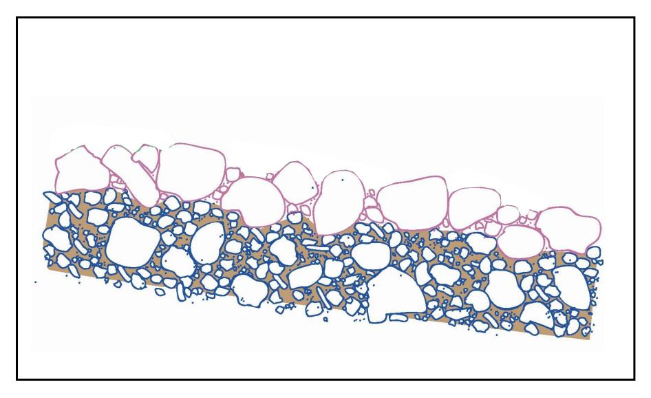
Figure 4.2-12. Illustration of an armored bed. As high flow releases from Shasta Dam transported gravels downstream, a greater proportion of the channel bed surface was covered by larger particles that could not be mobilized by high flow events. This armor layer traps gravels in the subsurface, making them unavailable for spawning.
