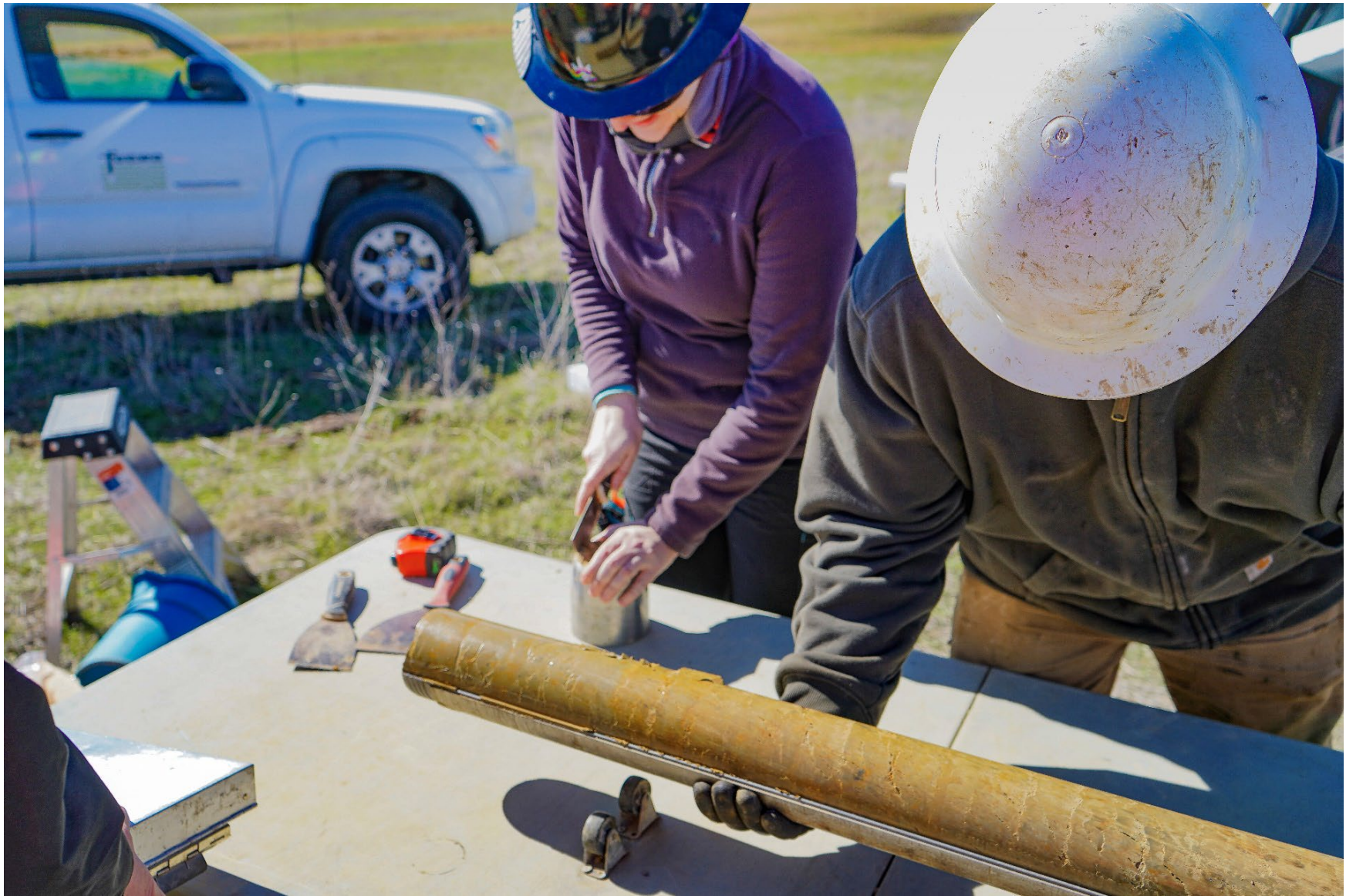
Photo 7 – Representative photo of crew reviewing collected core sample in the field.
