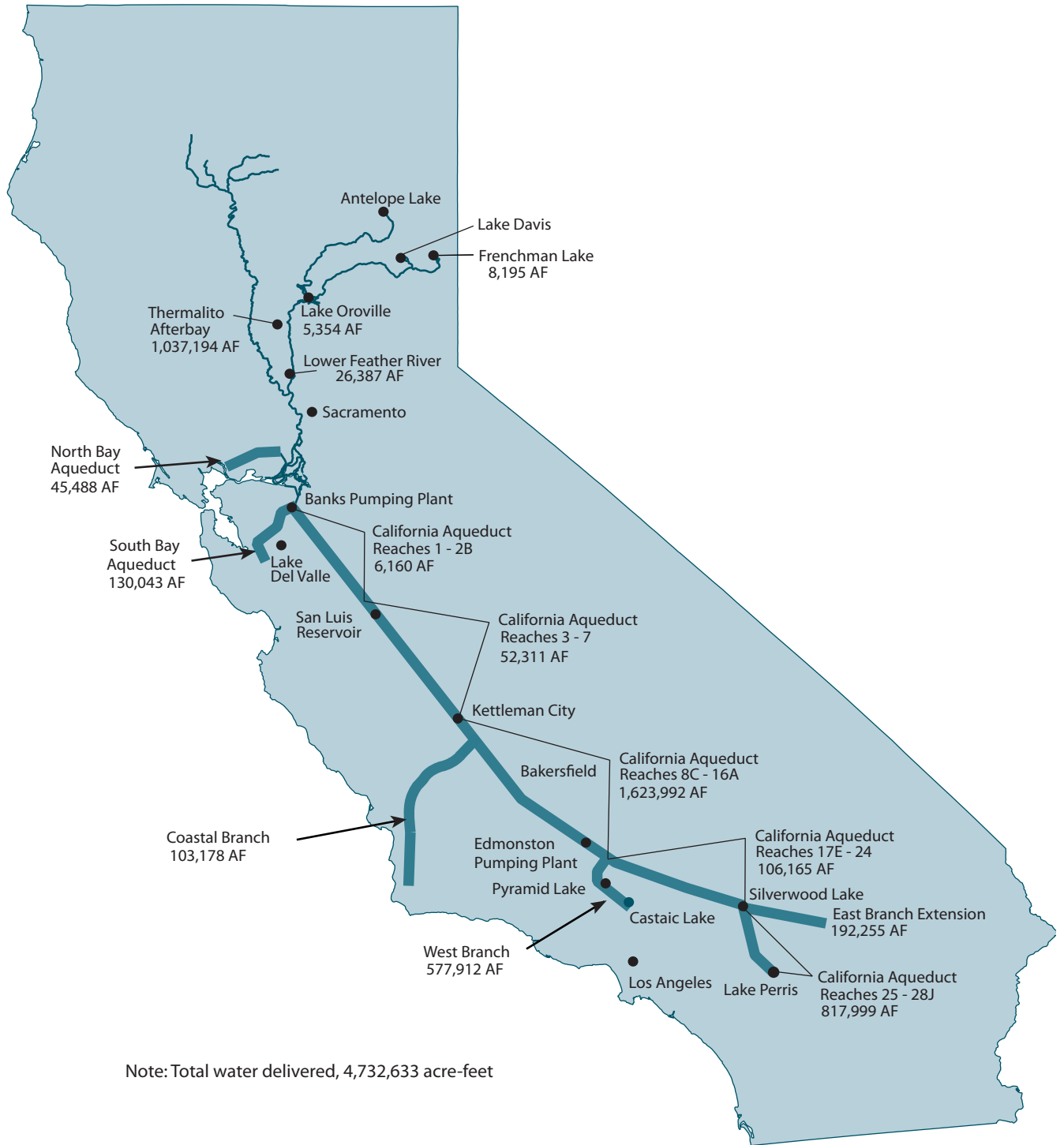
Figure 9-1. Water Delivered in 2005 and Delivery Locations of Long-Term Water Supply Contractors and Feather River Area Districts with Water Right Agreements with DWR
