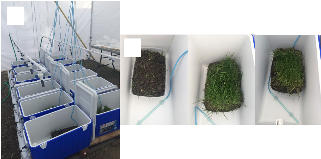
Figure 3-31 VegSens 2017 Mesocosm Experiment. Photos of (A) Mesocosm Chambers with Feed Water and Aeration Lines shown. (B) Disked, Grazed and Ungrazed Treatments (left to right, respectively)
