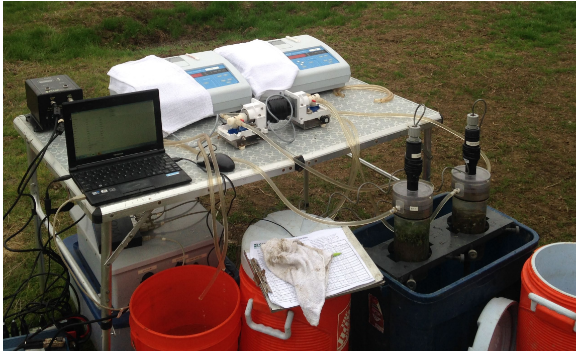
Figure 3-28 Photo of Sediment Erosion Study Experimental Setup in the Field Using Twin Gust Chambers (cylinders suspended above blue tub, lower right)
