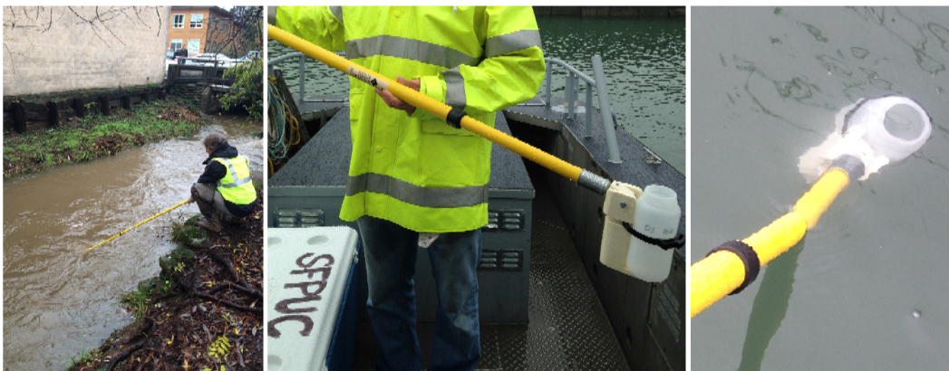
Figure 1. Nasco™ Swing Extension Sampler for taking grab samples of contaminated water sources
