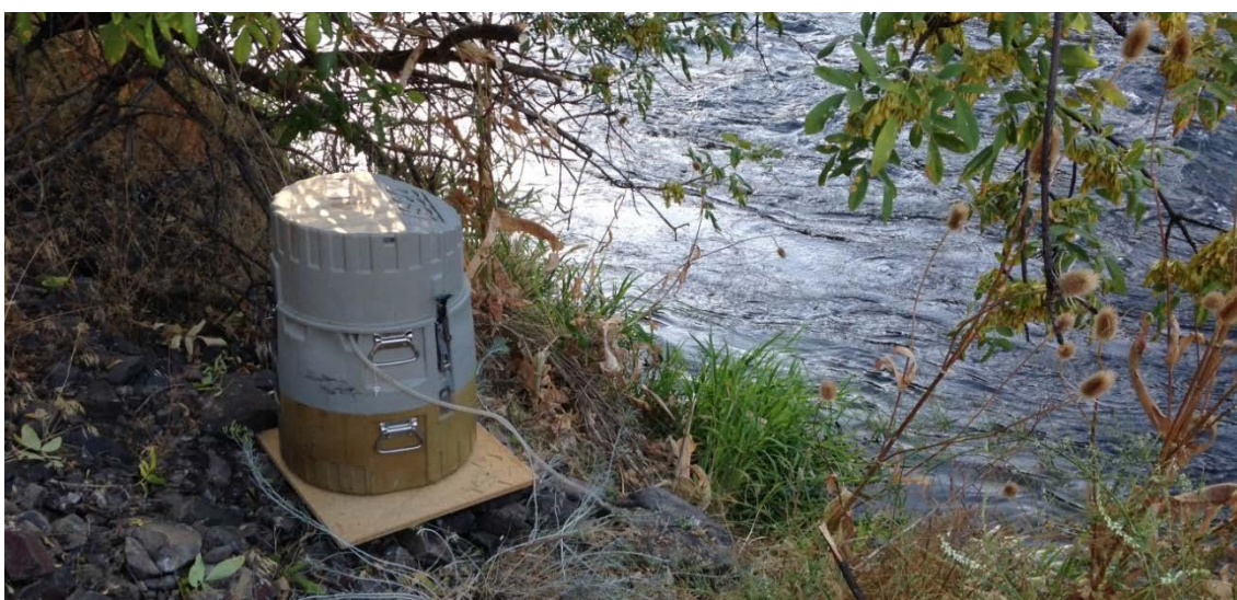
Figure 32. Autosampler Located Adjacent to the Klamath River Downstream of Iron Gate Dam.
