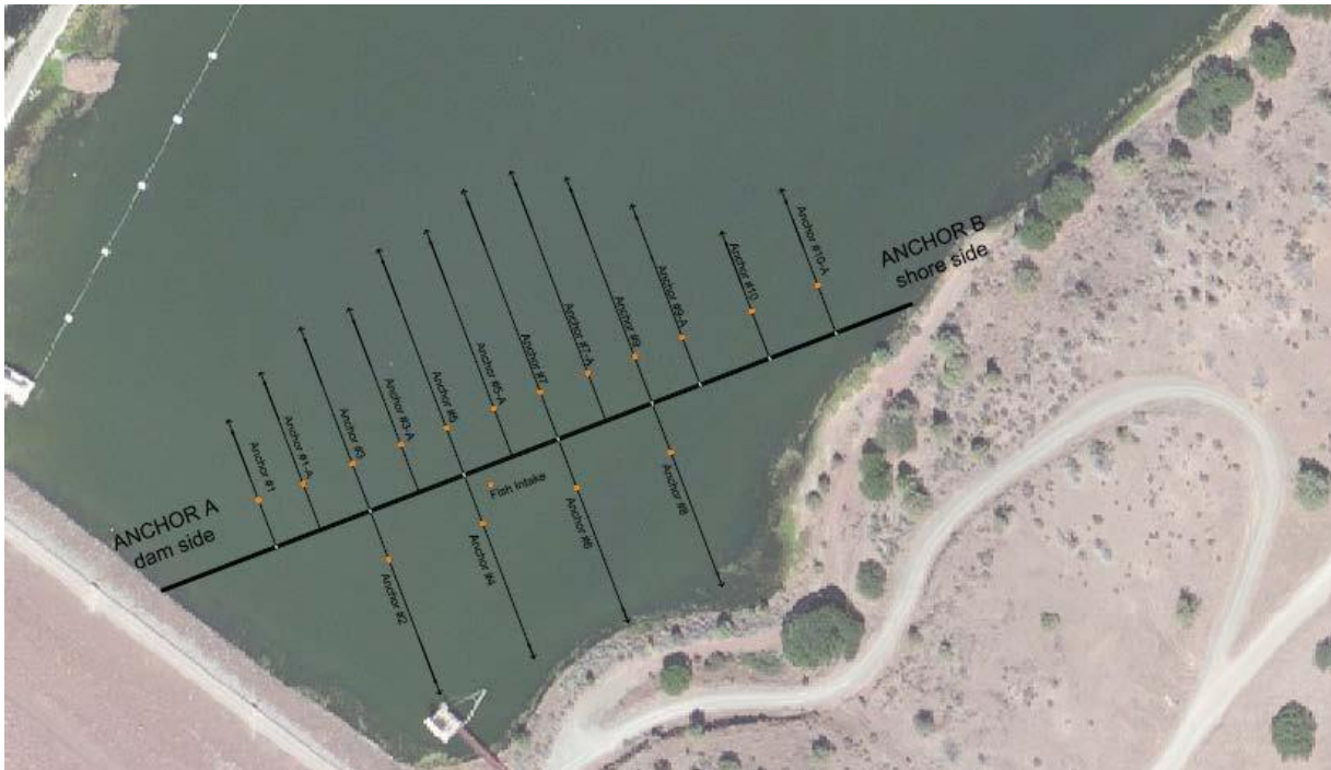
Figure 3. Plan View of Curtain Upstream of the Iron Gate Powerhouse Conduit Intake Near the Southeast Abutment of Iron Gate Dam.
