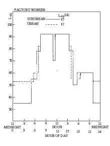
Figure B-3. Typical Noise Exposure Pattern of a Factory Worker<sup>B-1, B-4, B-8, B-9</sup>
