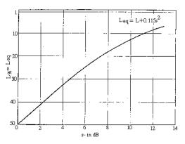
Figure A-5. Percentile of a Normal Distribution that is Equal to  $L_{eq}^{A-25}$  (See Equation A-14 and Probability Function).
