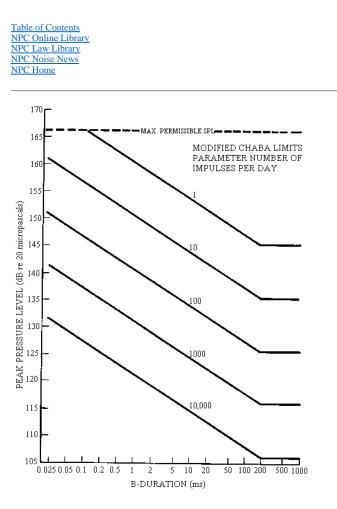
Figure 4. Set of Modified CHABA Limits for Daily Exposure to Impulse Noises Having B-Duration in the Range 25Microseconds to 1 Second. (Parameter: number (N) of impulses per daily exposure. Criterion: NIPTS not to exceed 5 dB at 4 kHz in more than 10% people.)
