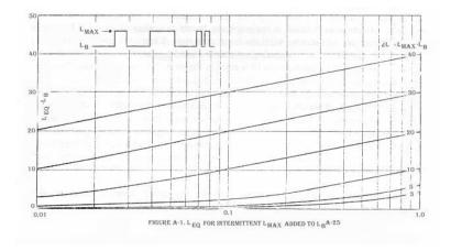
Figure A-1.  $L_{eq}$  for Intermittent  $L_{max}$  Added to  $L_b^{A-25}$ A-8
