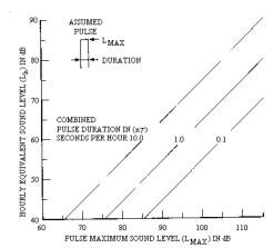
Figure A-3.  $L_{eq}$  for a Repeated Series of n Triangular Signals Overlaid on a Background Level of  $L_{b}$ , dB and  $\tau$ = Duration at ( $L_{max}$ -10) dB in Seconds.<sup>A-25</sup> (See Equation A-9).
