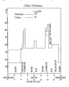
Figure B-4. Typical Noise Exposure Pattern of an Office Worker<sup>B-1, B-4, B-8, B-9</sup>
