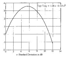
Figure A-6. Difference Between  $\rm L_{10}$  and  $\rm L_{eq}$  for a Normal Distribution  $\rm ^{A-25}$
