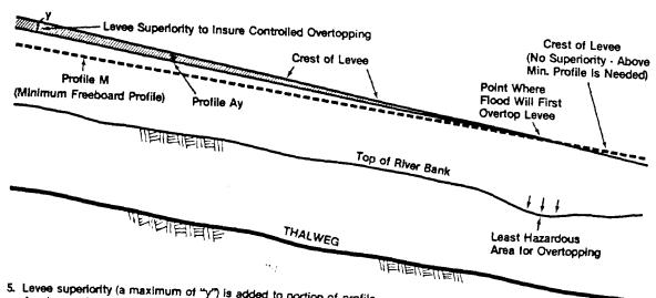
Levee superiority (a maximum of "y") is added to portion of profile Ay above minimum freeboard profile to assure overlopping first at least hazardous area.
