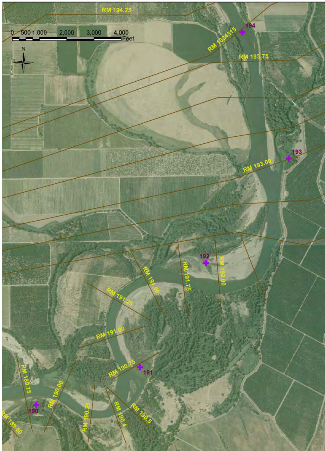
Figure 6-6. Comparison of CDWR (1991) and USACE (2002) river mile designations with overlap from RM 190 to RM 194. CDWR (1991) river mile designations are shown as purple crosses. Cross sections are from USACE (2002) study.
