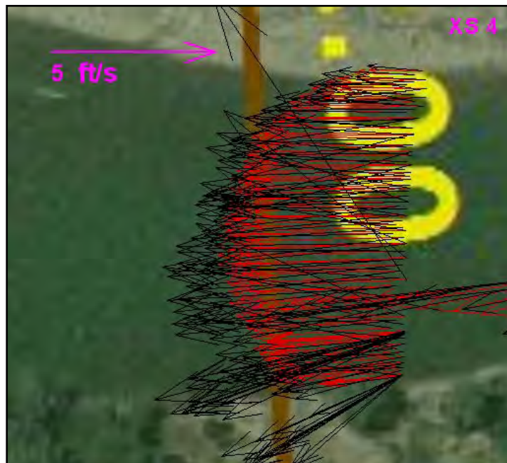
Figure 4-19. Comparison of velocity vectors at cross section 4 between measured and U 2 RANS data. Black arrows are computed and red arrows are measured.
