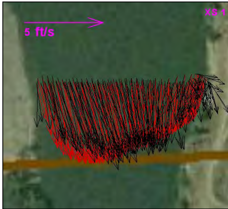
Figure 4-12. Comparison of velocity vectors at cross section 1 between measured and SRH-2D data. Black arrows are computed and red arrows are measured.
