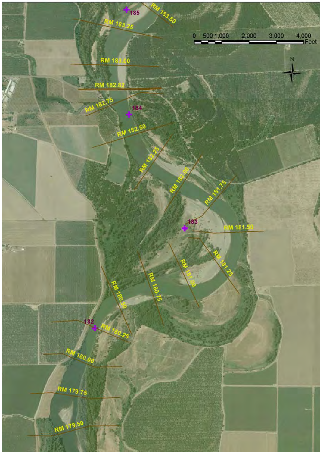
Figure 6-5. Comparison of CDWR (1991) and USACE (2002) river mile designations with overlap from RM 182 to RM 183. CDWR (1991) river mile designations are shown as purple crosses. Cross sections are from USACE (2002) study.
