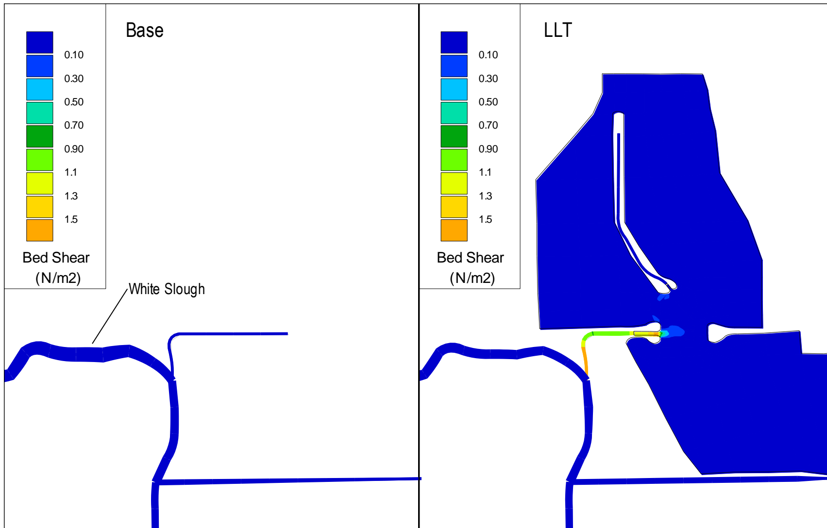
Figure 5-99 Bed shear near East Delta ROA for the Base case and LLT scenario during July 2002.
