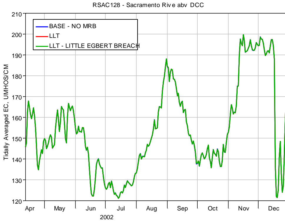
Figure 5-130 Tidally averaged EC at RSAC128 for Base-No MRB, LLT and LLT-Little Egbert Breach.
