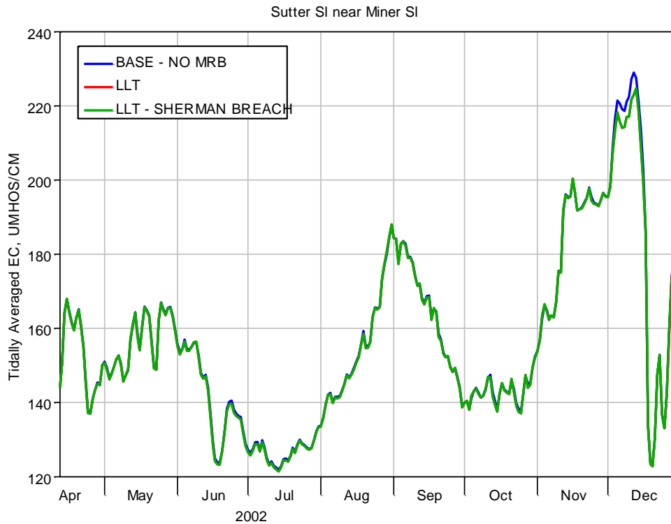
Figure 5-152 Tidally averaged EC in Sutter Slough for Base-No MRB, LLT and LLT-Sherman Breach.
