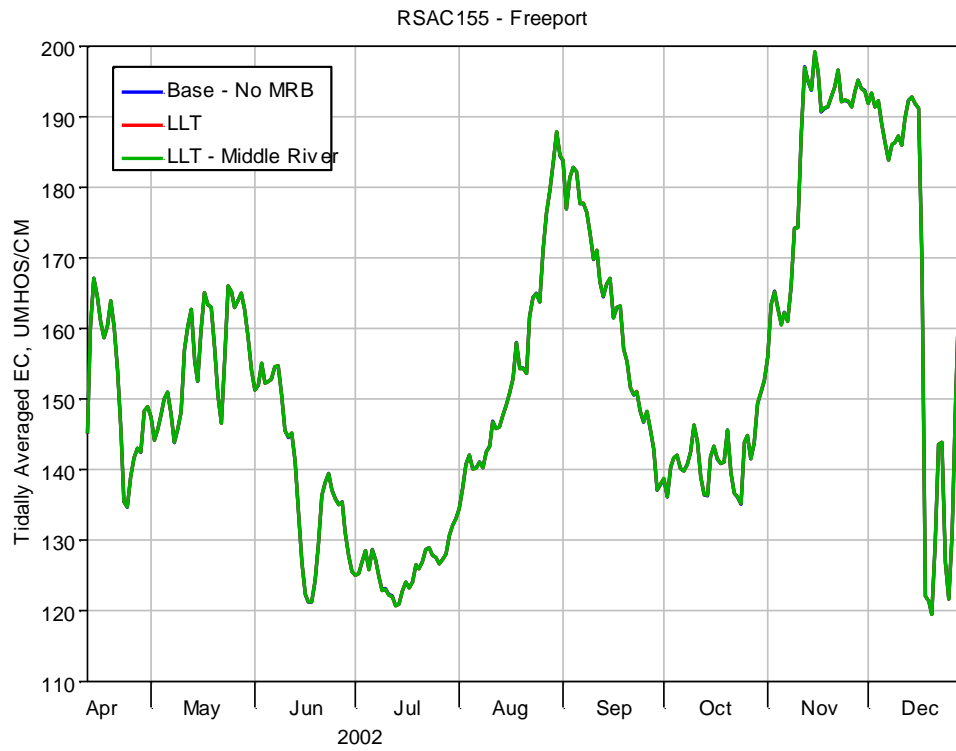
Figure 5-51 Tidally averaged EC at RSAC155 for Base-No MRB, LLT and LLT-Middle River.
