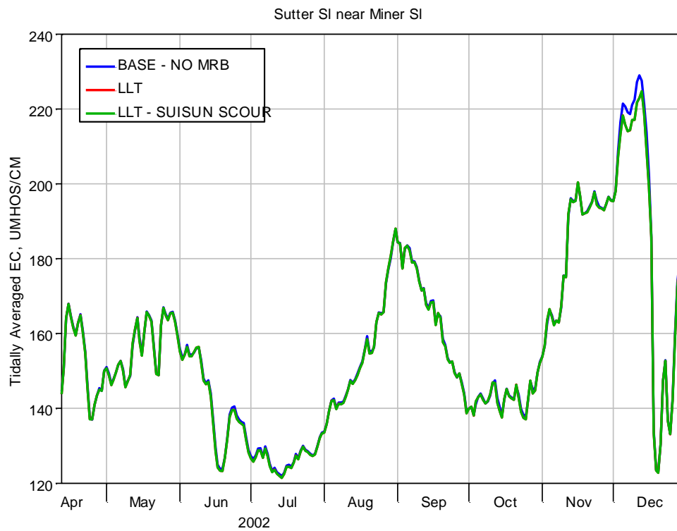
Figure 5-79 Tidally averaged EC in Sutter Slough for Base-No MRB, LLT and LLT-Suisun Scour.
