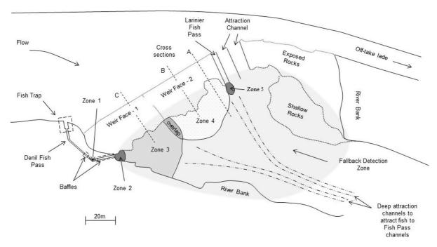
Fig. 2 Detail plan of obstacle structure and outline (grey shades) of detection zones. Also indicated are transects used to describe weir face
