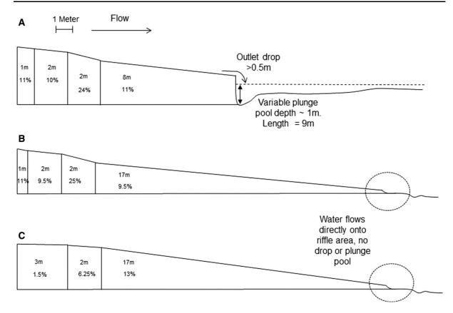
Fig. 3 Cross section of the weir transects identified in Fig. 2. These cross sections represent the three possible channel options for fish ascending the main face of the weir. The width (meters) and slope (%) are outlined for each downstream portion of the weir face
