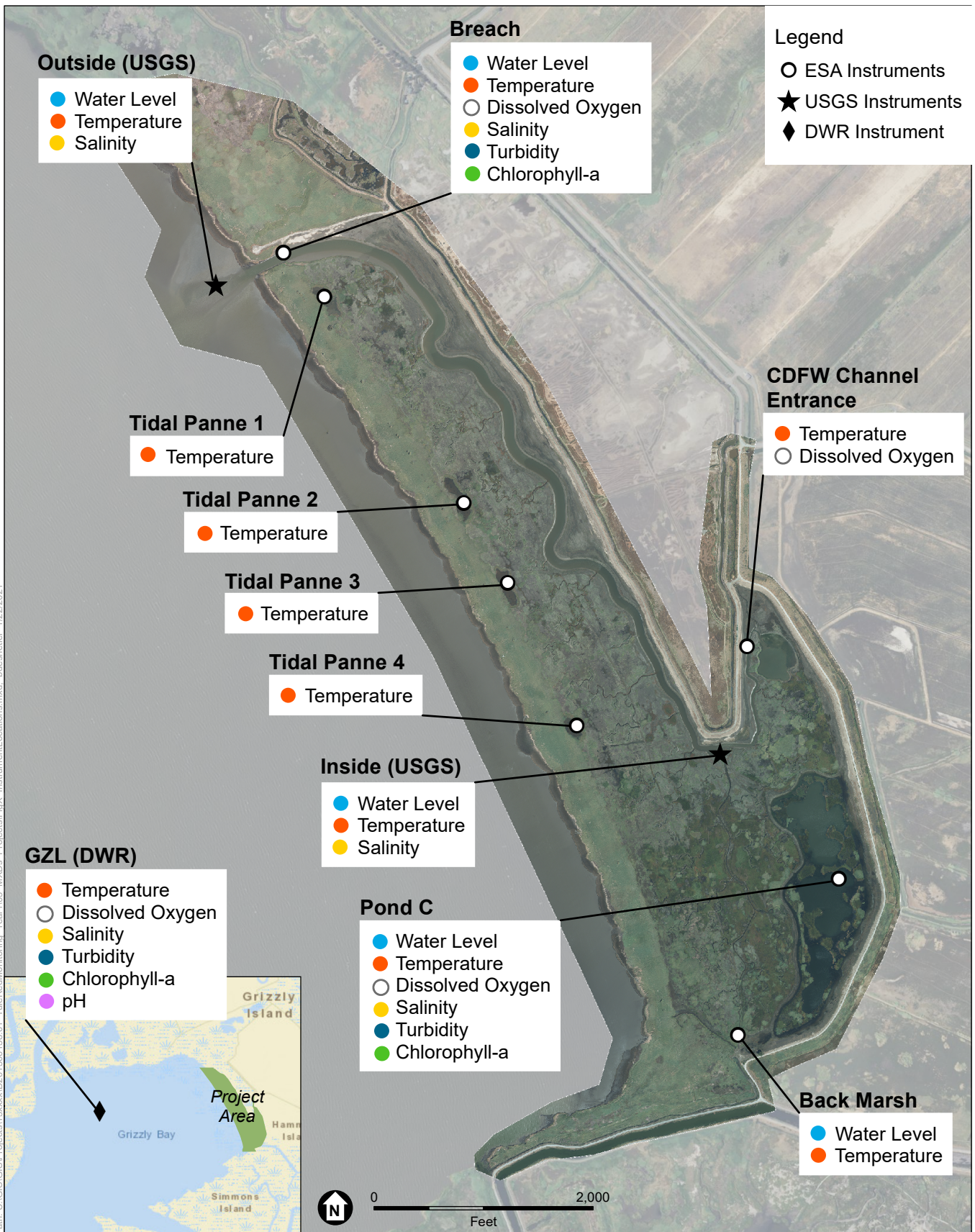
Figure 3-2 Water Quality and Water Level Instrument Locations
