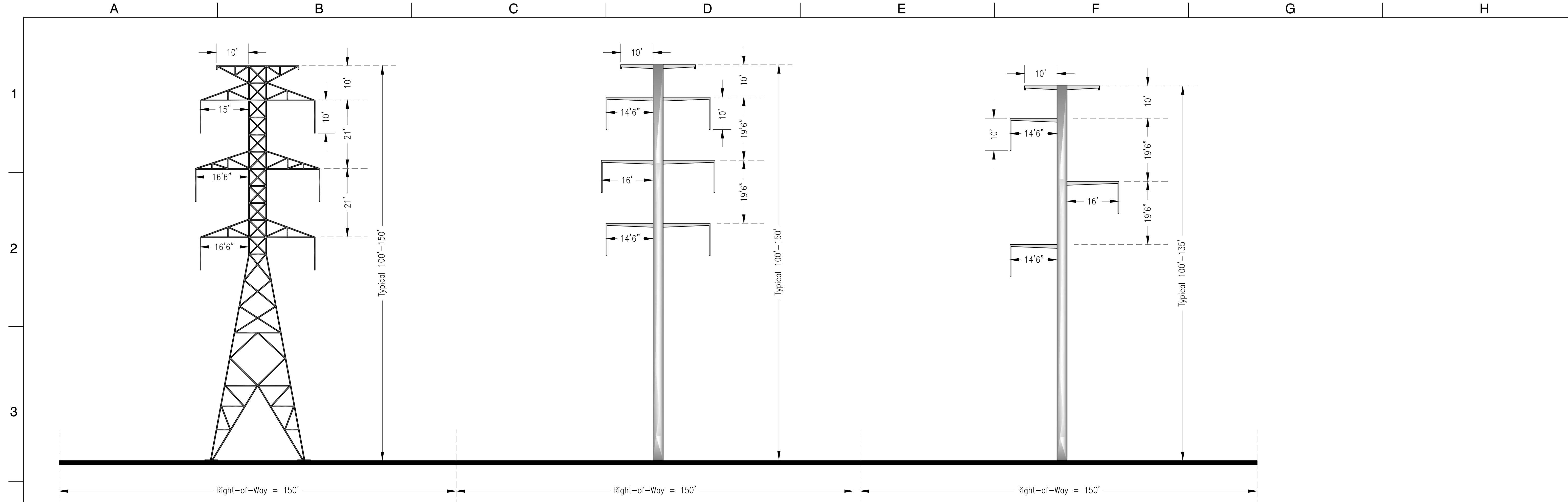
230kV DOUBLE CIRCUIT LATTICE STRUCTURE SCALE: NTS
