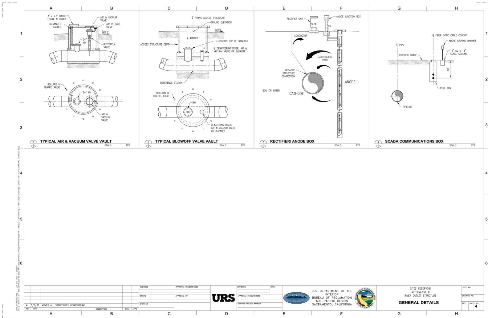
Figure B.3-40. Typical Pipeline Air Valve and Blow-off Details
