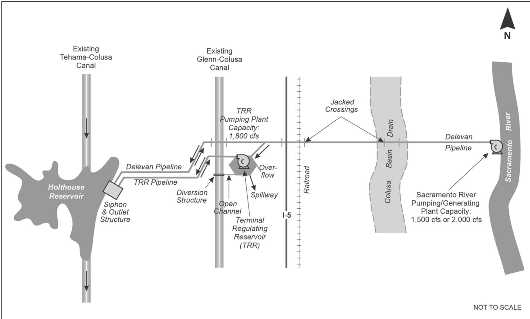
Figure B.3-41. Schematic Layout of New Sacramento River Conveyance Delevan Pipeline
