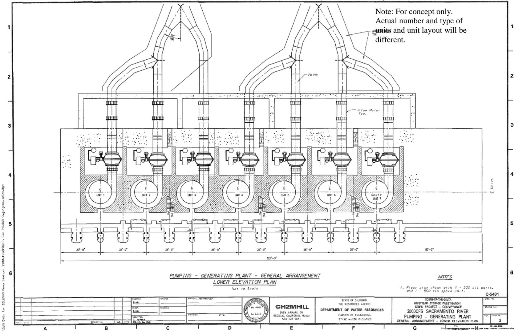
Figure B.3-44. Sacramento River Pumping/Generating Plant Lower Elevation Plan
