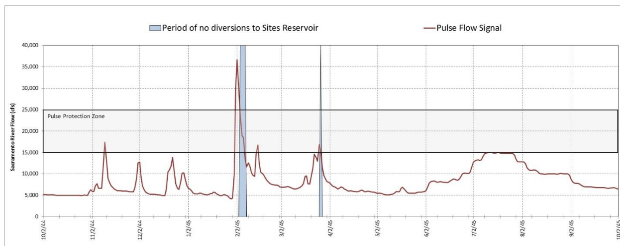
Figure D.3-2: Example of Sacramento River Pulse Protection Zone and periods of no diversions to Sites Reservoir during Pulse Conditions
