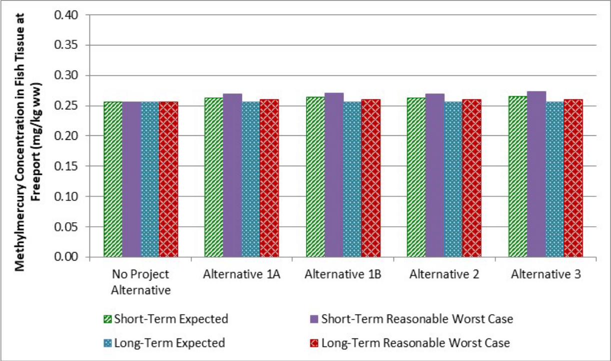
Figure 6-7. Estimated Fish Tissue Methylmercury Concentrations at Freepoint for the No Project Alternative and Alternatives 1, 2, and 3 for Annual Average Flows.
