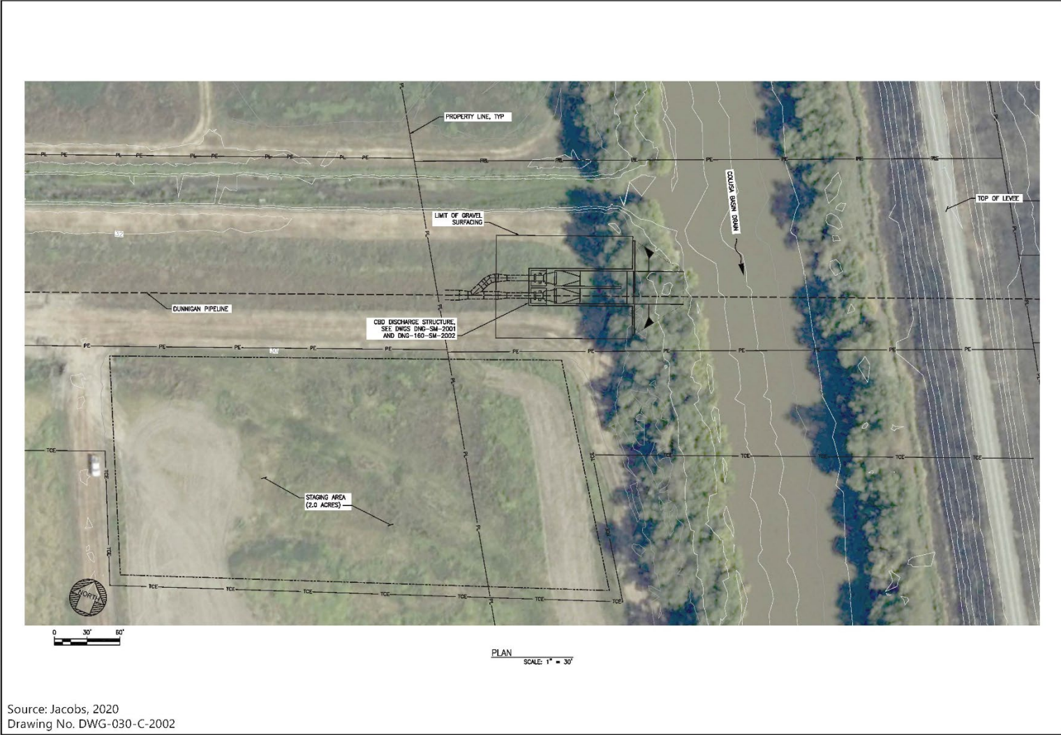
Figure 2-33. Dunnigan CBD Discharge Site Plan
